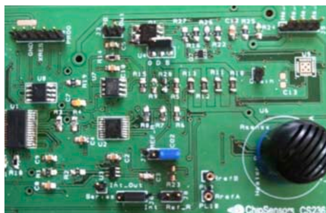
Generic Microcontroller PCB with CO 2 gas sensor
