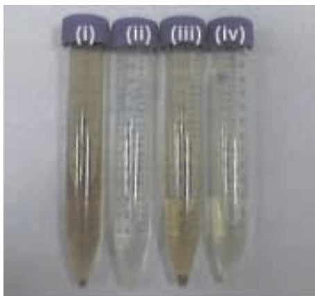
Figure 3.27. Visual of extraction of pollutants within the industrial sample. (i) Original industrial sample, (ii) filtered through Si-NH, (iii) filtered through Si-SH, and (iv) filtered through SH-Si-NH.
