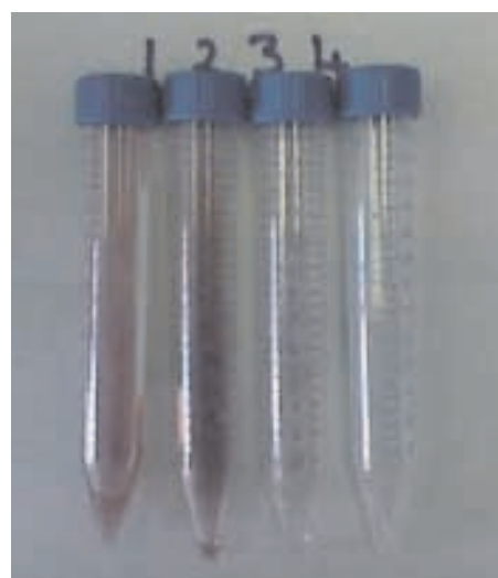
Figure 3.29. Visual absorbance of (1) standard gold nanoparticles, (2) post-Si-NH extraction, (3) post-Si-SH extraction, and (4) post-Si extraction.
