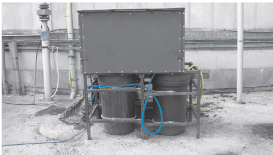
Figure 2.2. Photo of the pilot-scale sequencing batch reactor showing the reactor tank (on left) and the holding tank (on right).
