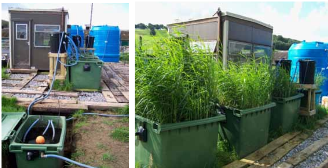
Figure 6.1. Layout of the pilot-scale field alum sludge-based constructed wetland system.
