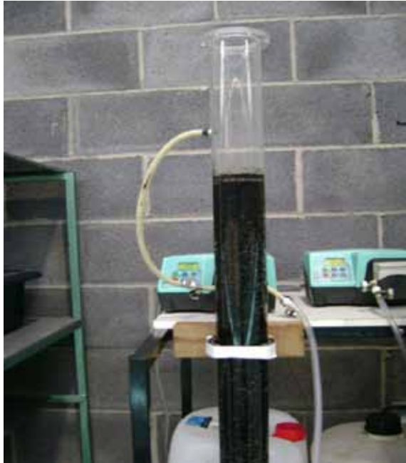
Figure 8.11. Continuous flow test system for polymer-release monitoring.
