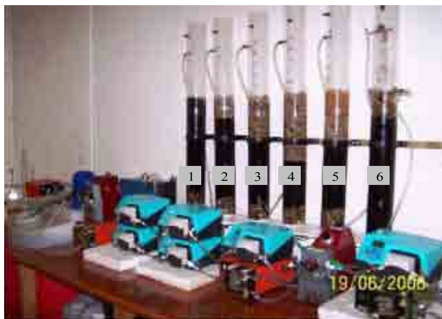
Figure 3.3. Laboratory-scale vertical flow constructed wetland reactors filled with different proportions of dewatered alum sludge.
