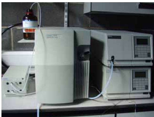
Figure 8.9. Photograph of the Waters HPLC used in this study.
