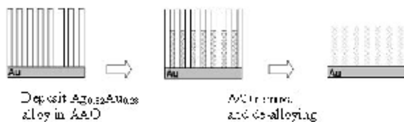
Fig 3.7. Route to fabrication of free-standing array of nanoporous gold wires.
