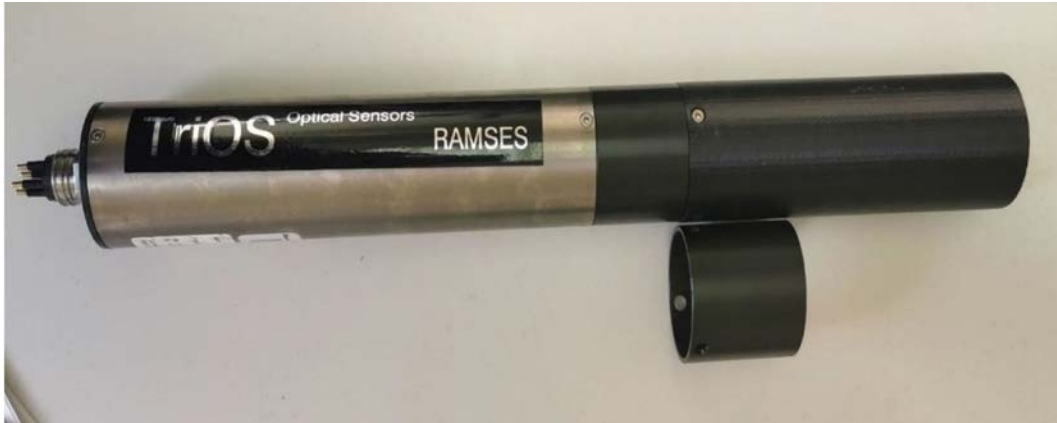
Figure 3.3. TriOS ARC-VIS RAMSES radiometric sensor showing the original black 5 cm tube and the newly fabricated 12 cm tube, which was found to be more effective under the normally relatively windy conditions often experienced in Ireland.
