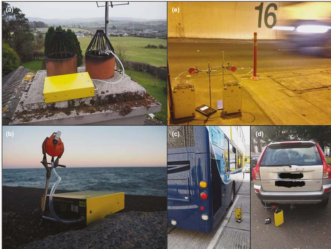
Figure 2.3. Direct PM_{2.5} source sampling set-up. The typical set-up for sampling PM_{2.5} sources, directly from source, using a conical inhalable sampler and a Casella Vortex Ultra Flow sampling pump. The PM_{2.5} sources sampled include (a) solid fuel emissions, (b) sea spray, (c) Dublin Bus exhaust emissions, (d) passenger vehicle exhaust emissions and (e) traffic emissions from inside the Dublin Port Tunnel.
