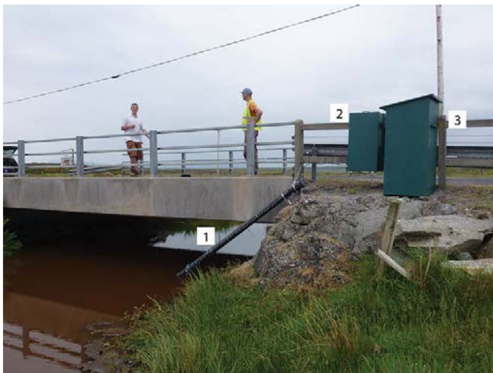
Figure 6.4. Monitoring site set-up showing (1) the PVC pipe housing the EXO2 sonde, (2) the custom-made box housing the Storm 3 data logger and (3) the box housing the ISCO autosampler.
