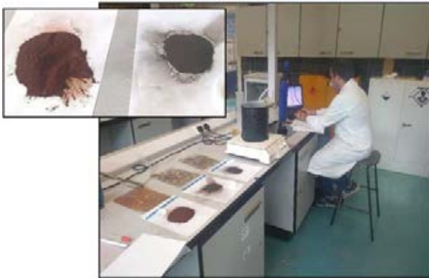
Figure 6.6. Laboratory set-up for the preparation of the in-house standards. Inset shows close-up of the two sediment types with Fe-rich sediment on the left.
