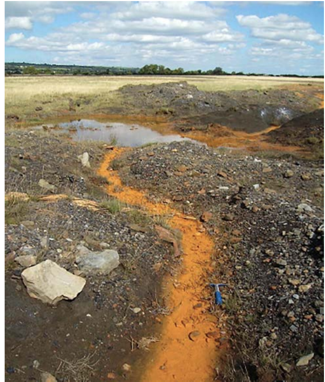
Figure 1.1. Example of AMD generation and colour leachate. Source: S. Callery.
