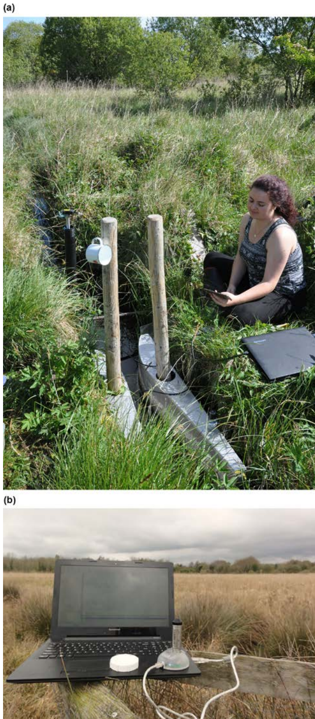
Figure 2.3. (a) Flume and level data logger installed at the outlet to Ballymore fen (Co. Westmeath) and (b) level logger (diver) being downloaded to field laptop.
