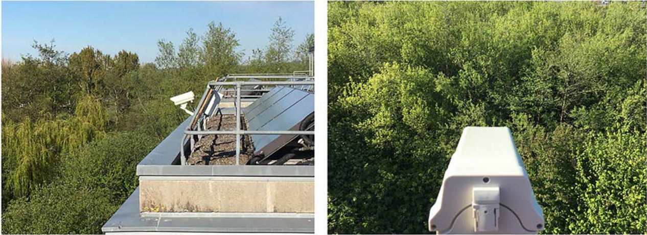
Figure 2.1. Phenocam (StarDot NetCam SC) pointed at a tree canopy in Cork. For information on the use of phenocam images see Chapter 4. Photos: Calum Sweeney.
