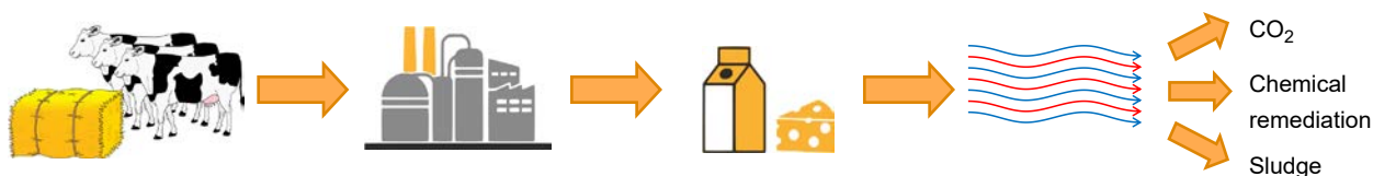
Figure 1.1. The linear dairy processing system. The processing of milk into dairy products creates wastewater, which is remediated using chemical processes, releasing CO 2 and creating sludge.
