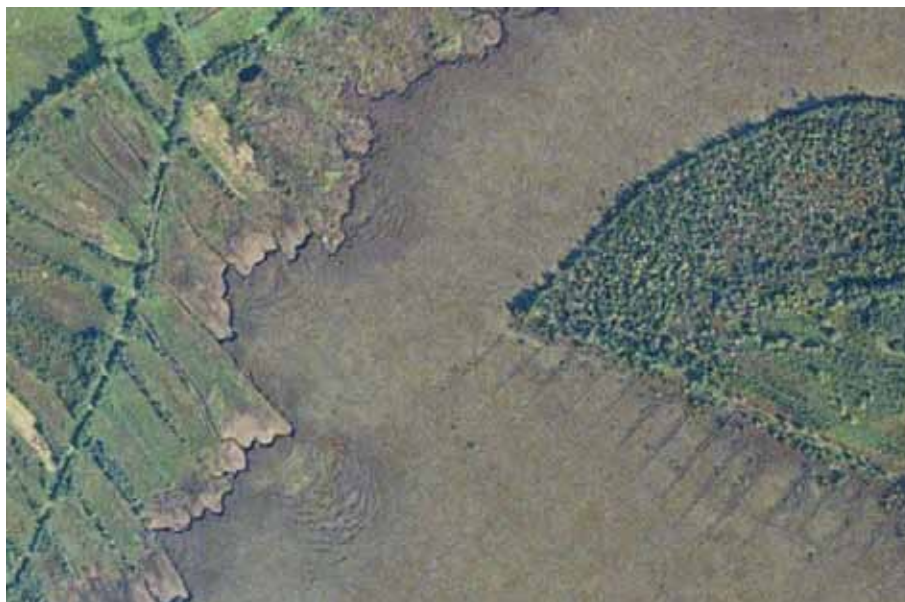
Figure 2.10. Section of 2005 aerial photograph of Carn Park bog showing northern failed area (courtesy Charise Mc Keown, Geological Survey of Ireland).
