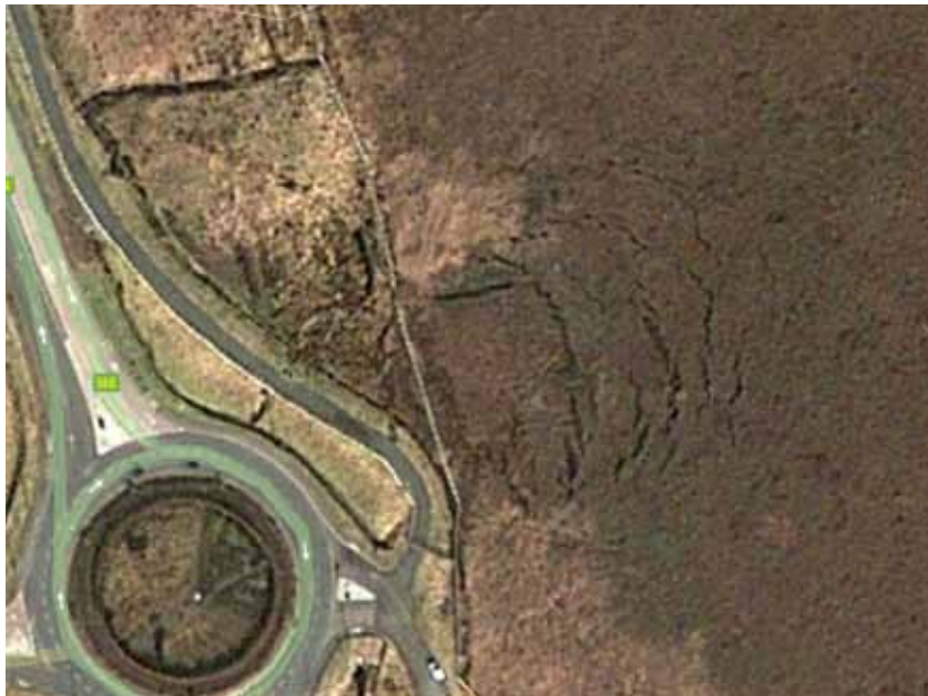
Figure 2.13. Image showing failed section of Aghnamona Bog, Roosky. Imagery © DigitalGlobe, Map data © Google.
