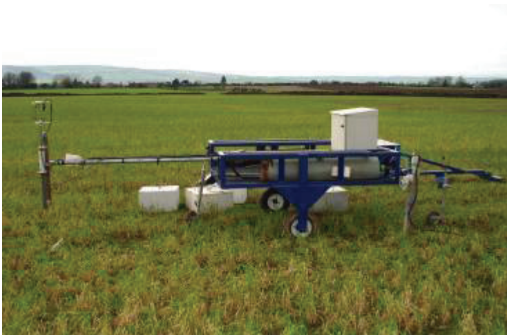
Figure 2.2. The closed path eddy covariance system mounted on the mobile trailer.
