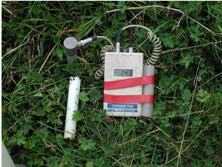
Figure 4.14 Tensiometer monitoring soil moisture potential below a percolation trench. The tensiometer cover can be seen to the left of the tensiometer.
