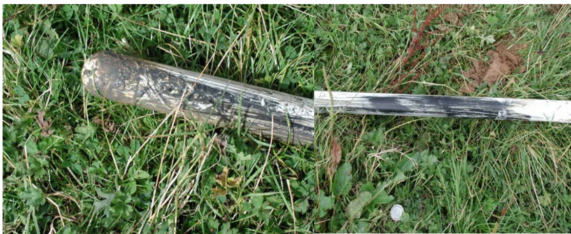
Figure 5.7 (a) and (b) Biofilm build-up on preferential flow lysimeters.
