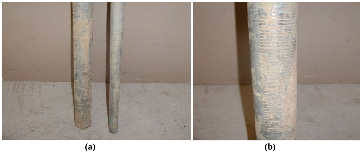
Figure 4.13 (a) Large and small bore zero tension samplers and (b) clogged large bore sampler.
