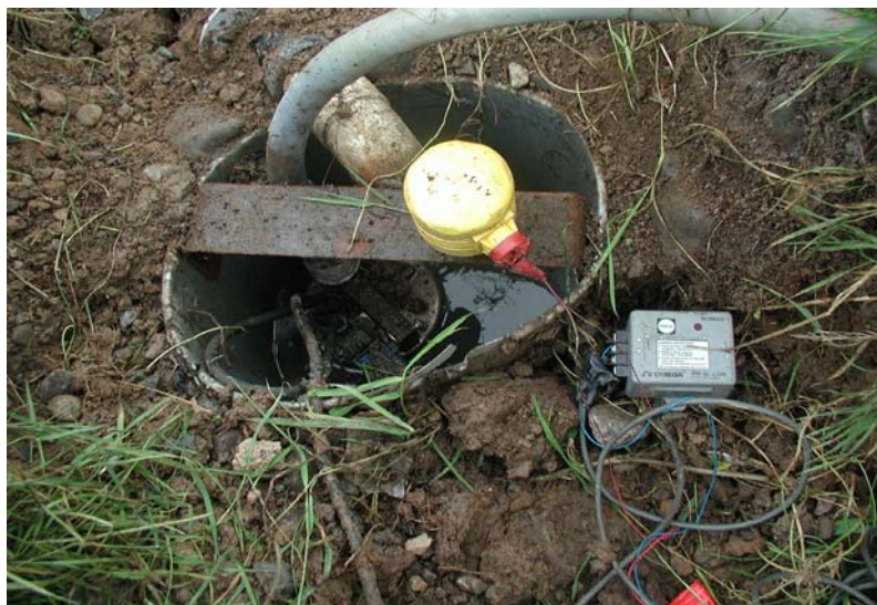
Figure 4.5 Septic tank effluent flow measurement on Site 1.
