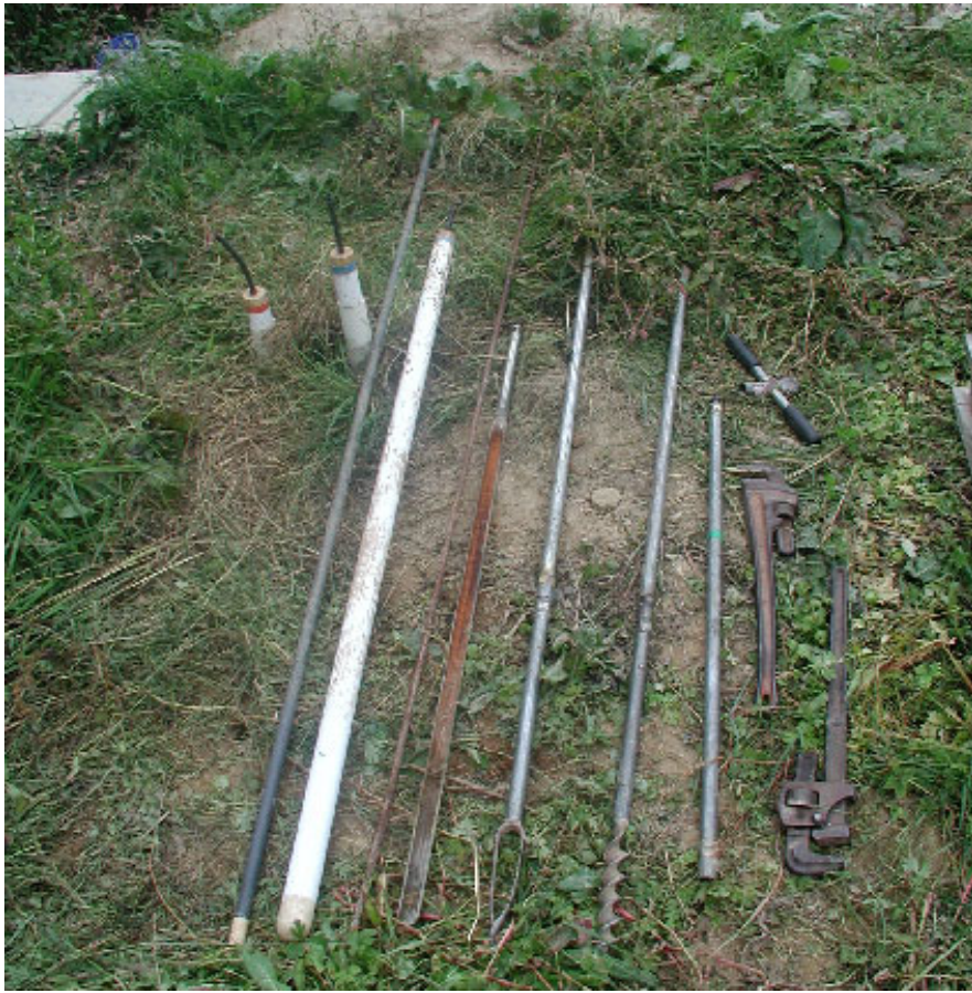
Figure 4.8 Percolation trench monitoring instrumentation and equipment required for its installation. From left of photograph: 2.0m tensiometer, 1.6m lysimeter, steel reinforcing bar, gouge auger, combination auger, screw auger, auger extension bar, auger handle and stilson wrenches.
