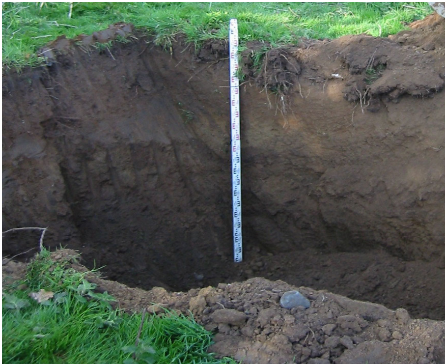
Figure 2. 7 Trial hole on Site 2.
