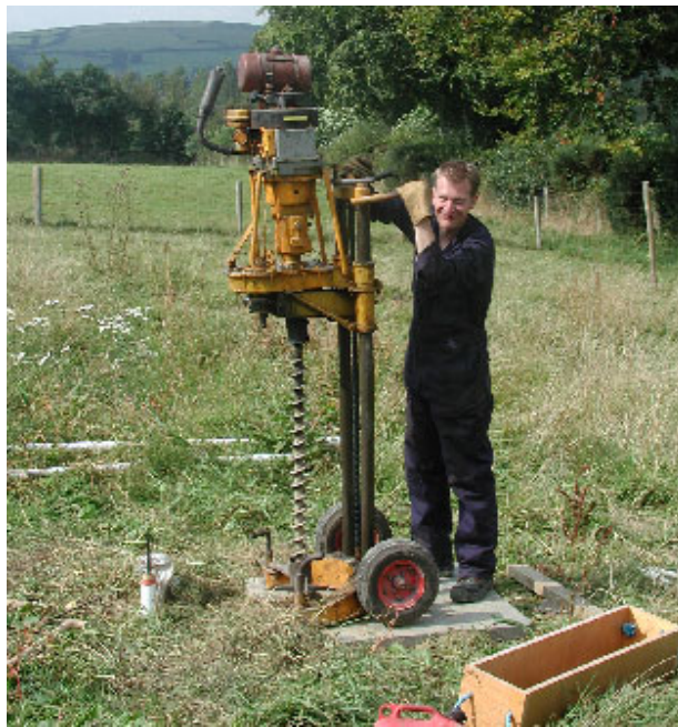
Figure 4.10 Installation of lysimeters using the Minute Man.
