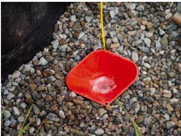
Figure 3.11. Installation of gravity samplers in sand filters.
