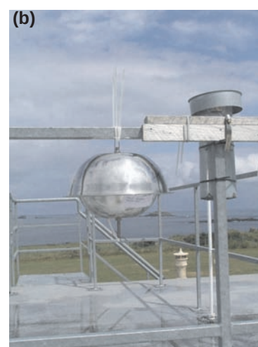
Figure 8.1. (a) Sites for passive samplers for the Global Atmospheric Passive Sampling (GAPS) study; (b) passive persistent organic pollutant (POP) sampler at Mace Head.
