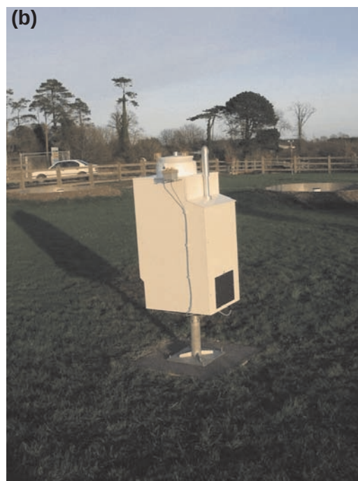
Figure 3.4. Carnsore Point site (a) and associated precipitation sampler in Wexford (b).
