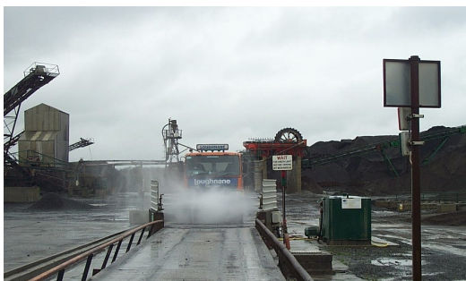
Wheelwash Facility (Loughnane Concrete, Birr, Co. Offaly)
