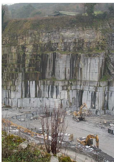
Extraction of dimension stone (McKeon Stone, Threecastles, Co. Kilkenny)
