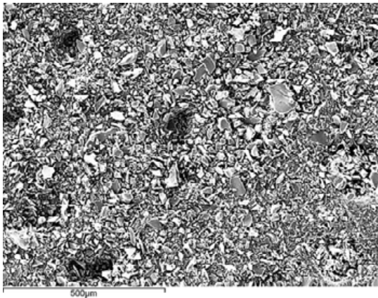
Figure 3.17. C2-M3-GB SEM image showing GB particles filtered through a 53 µm filter after bulk grinding.
