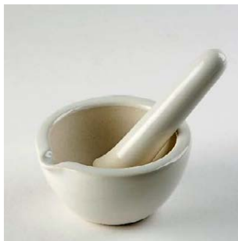
Figure 2.2. Mortar and pestle used to crush the GB and GF samples.
