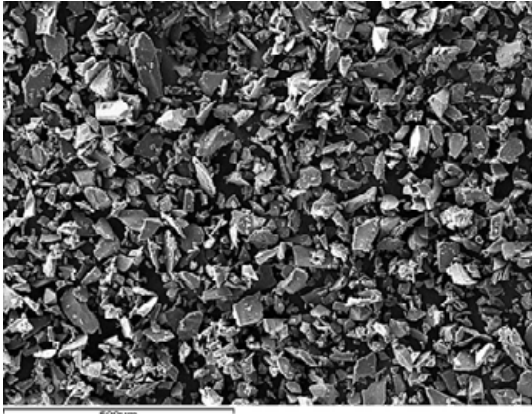
Figure 3.12. C2-M3-GF SEM image showing GF particles filtered through a 53 µm filter after bulk grinding.
