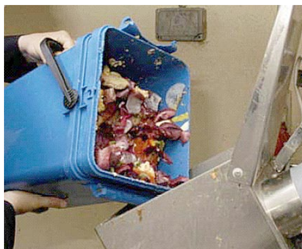
Figure 2.10: Hotel Food Waste Disposed of in Compactor and Dewaterer
