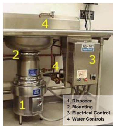
Figure 2.4: Functional Parts of a Commercial FWD
