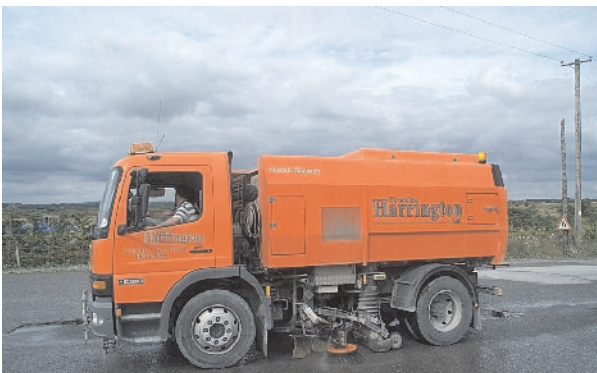
Figure 4.1. Vacuum road sweeper (Frank Harrington Ltd, Co. Mayo).
