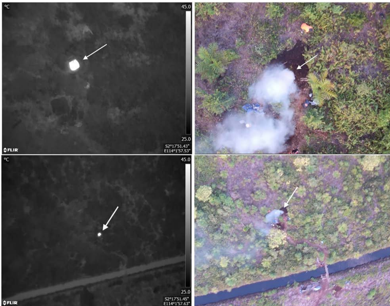
Figure 1.3. Thermal infrared image taken from a drone showing a thermal image of a peat fire (left) and a true colour image of the same fire (right). Reproduced from Burke et al. (2019); licensed under CC BY4.0 ( https://creativecommons.org/licenses/by/4.0/ ).
