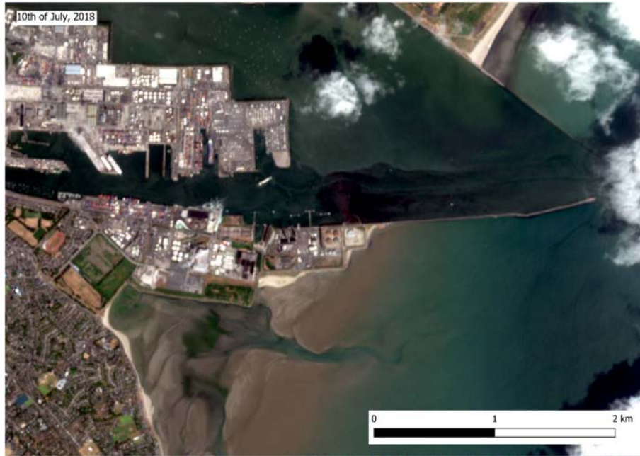
Figure 3.1. Sentinel-2 image showing discharge from Ringsend WWTP on 10 July 2018. A large dark trail can be seen exiting the harbour with a reddish discharge emanating from the WWTP.
