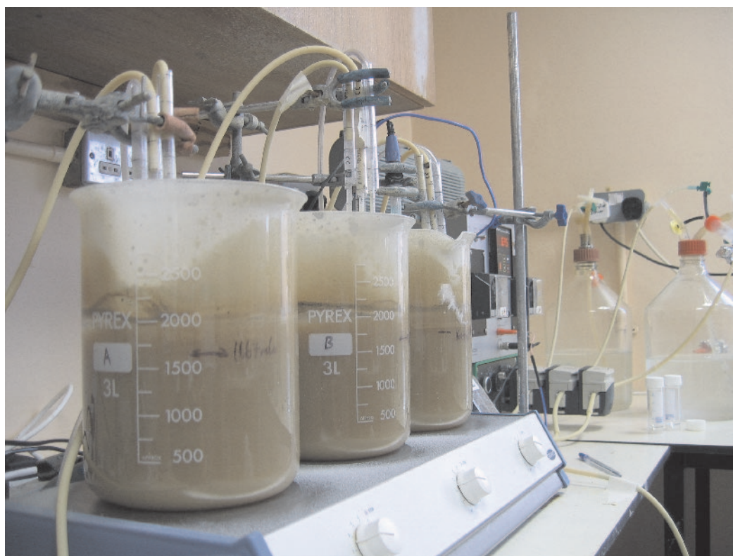
Figure 3.2. Sequencing batch reactor set-up for acid-shock work.
