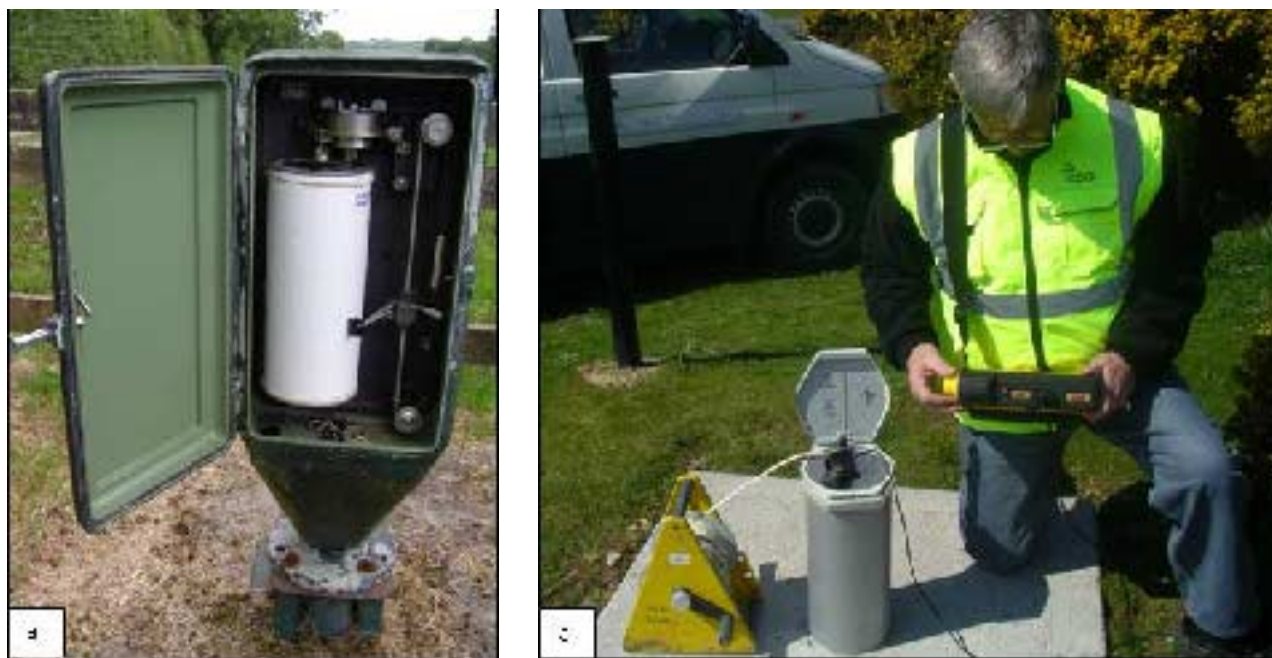
Figure 6.1. Groundwater level monitoring systems. (a) Geological Survey of Ireland chart recorder recording groundwater levels. (b) Downloading groundwater level data from a digital logger at an Environmental Protection Agency Water Framework Directive monitoring point.
