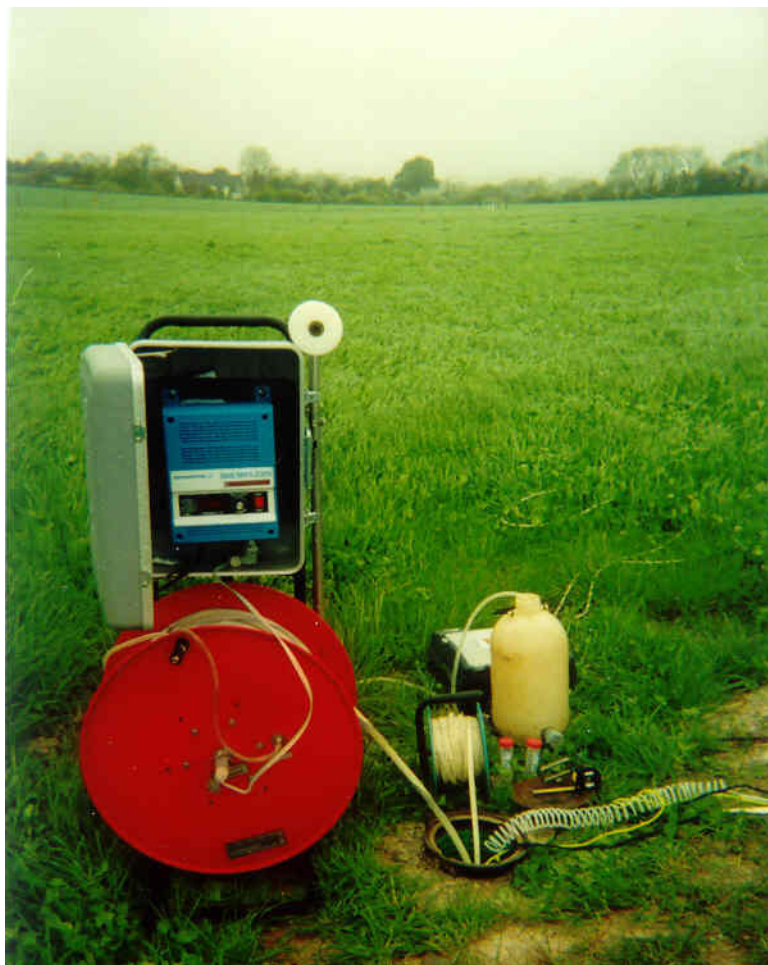
Figure B.3 Sampling set-up at a Curtin's farm borehole (generator not shown).
