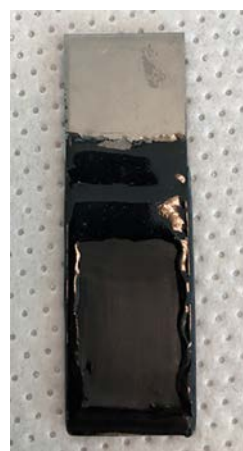
Figure 3.29. Photograph of the screen-printed carbon-based electrode tested as a feeder electrode in the SPy reactor.
