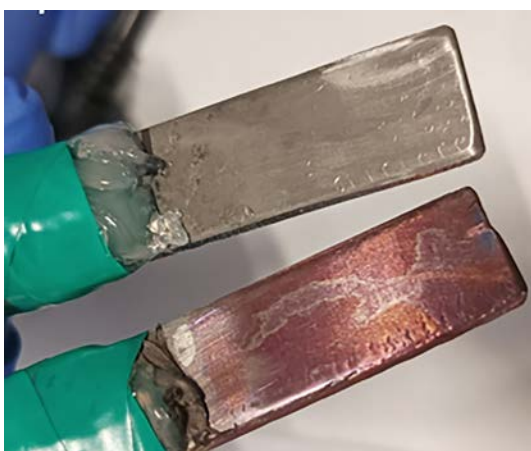
Figure 3.28. Upper electrode is a pristine titanium electrode and the lower electrode is a titanium electrode following oxidation at +1.8V for 300 s.
