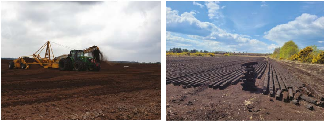
Figure 1.1. Left: cutaway peatland (historical industrial extraction by Bord na Móna at Coolcraff, Co. Longford, 2020). Right: cutover peatland (domestic extraction by private contractors using the “sausage” technique at Ballydaly, Co. Offaly, 2021). Source: Florence Renou-Wilson.
