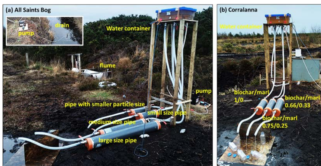
Figure 4.7. Experimental setups in (a) All Saints and (b) Corralanna, where effluent treatment in pipe-encased biochar was tested at the outlets of the catchments.
