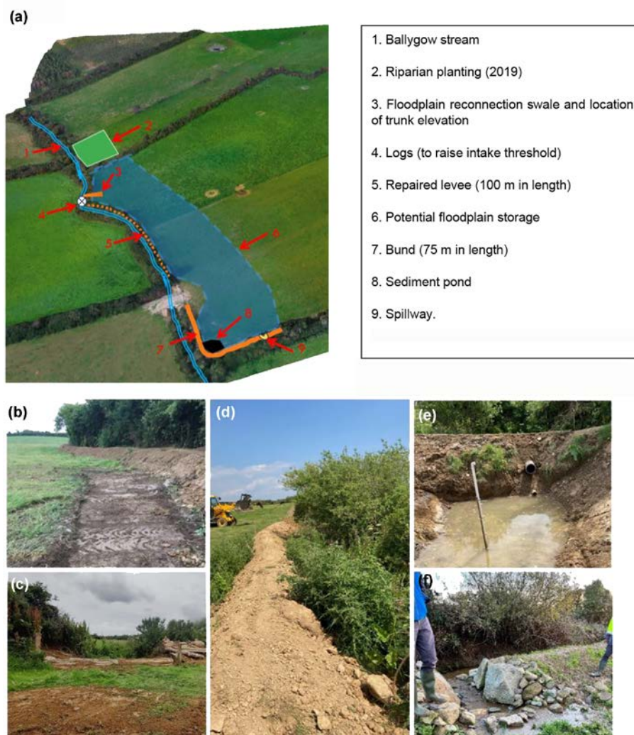
Figure 2.1. Site 1: Ballygow, Co. Wexford. Panel (a) shows the demonstration site and its features; panel (b) shows the floodplain reconnection swale and location of trunk elevation; panel (c) shows logs (to raise intake threshold); panel (d) shows the bund (75 m in length); panel (e) shows the sediment pond; and panel (f) shows the spillway. For a detailed description, see www.slowaters.eu .
