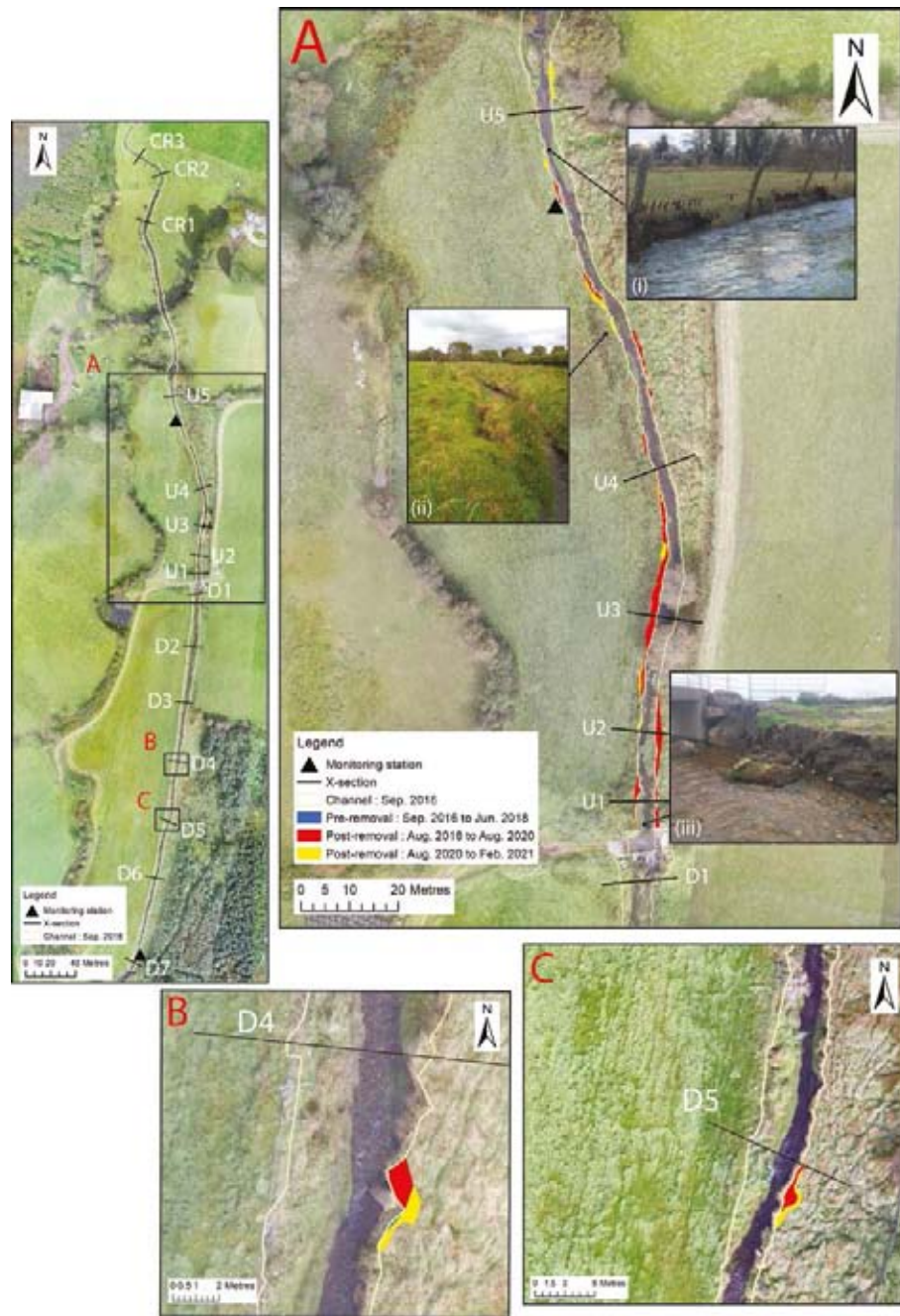
Figure 6.10. Planform adjustments at Browns Beck Brook between September 2016 and February 2021. The locations of panels A, B and C are shown in panel the site map (top left). Inset photos in panel A correspond to (i) linear erosion along a fence line above the upstream monitoring station in February 2018; (ii) slab failure in BBB-US in September 2020; and (iii) failure of cohesive banks immediately upstream of the new structure in September 2019.
