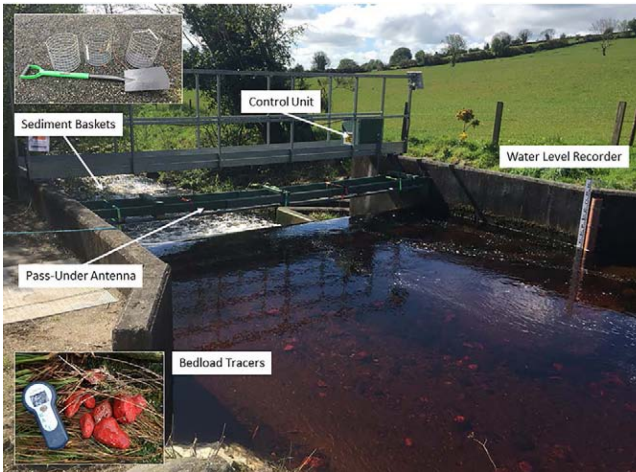
Figure 6.6. Study site showing the locations of the pass-under stationary antenna, water level recorder, control unit and bedload tracers. Reproduced from Casserly et al. (2021a); licensed under CC BY 4.0 ( https://creativecommons.org/licenses/by/4.0/ ).
