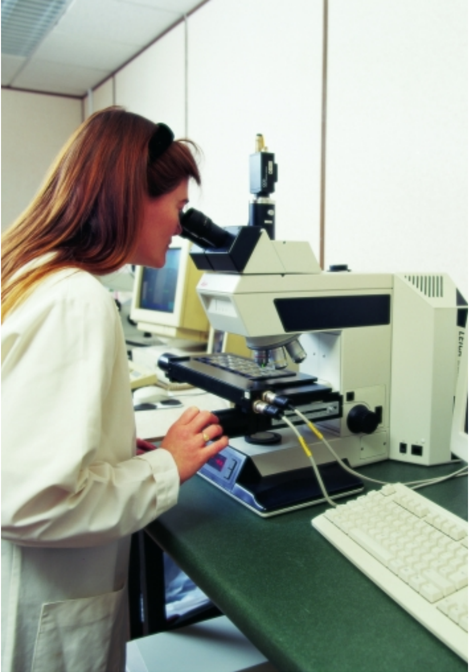
Radon concentration is determined by analysing the detectors under a microscope.
