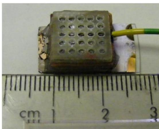
**Figure 1** Side view of Direct Borohydride Fuel Cell
