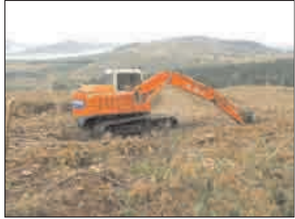
Figure 3.9. The Fiat-Hitachi FH130-3 excavator used. in collecting forest residuals into windrows.
