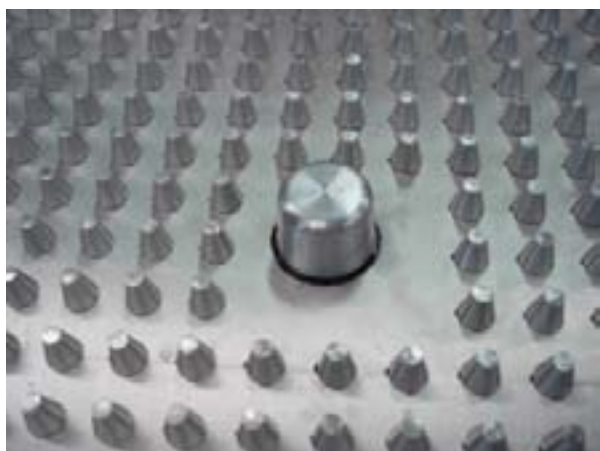
Figure 6.4. Aluminium vacuum mould for acrylonitrile butadiene styrene sheets.
