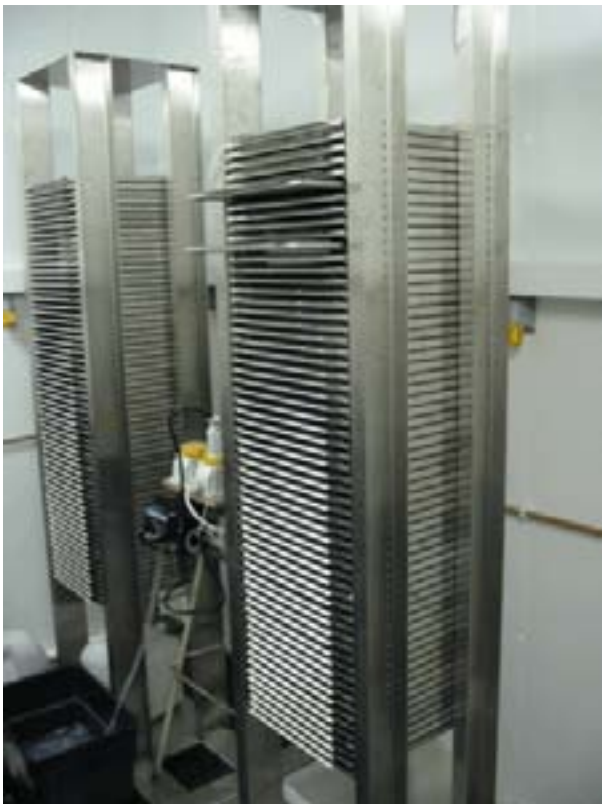
Figure 6.2. Laboratory horizontal flow biofilm reactor units.
