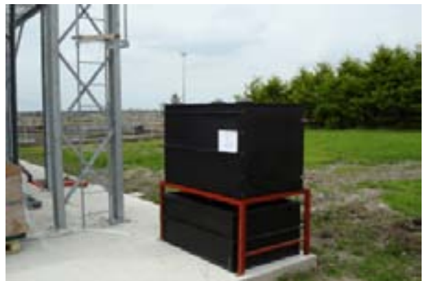
Figure 6.3. Horizontal flow biofilm reactor at Tuam Water Research Facility.
