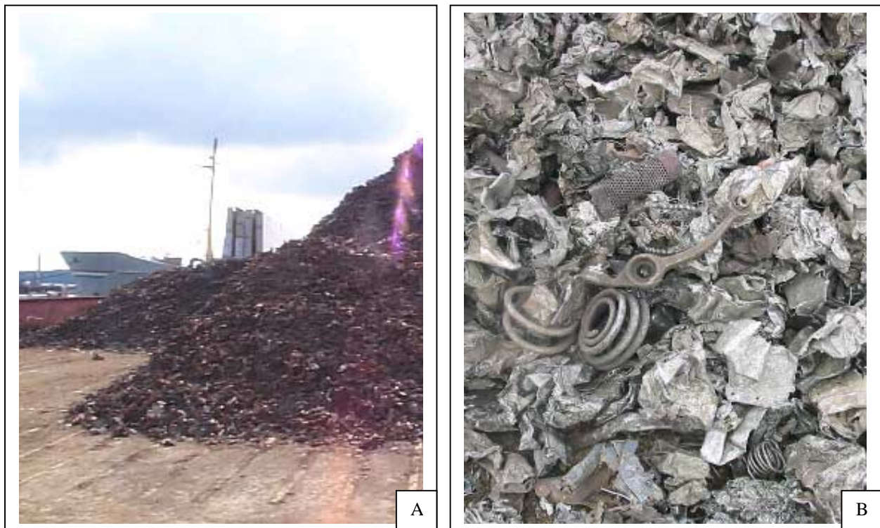
Photo 7 Shredded ferrous metal at Clearway, Belfast – A: Awaiting shipment; B: Close-up view of shredded ferrous metal
